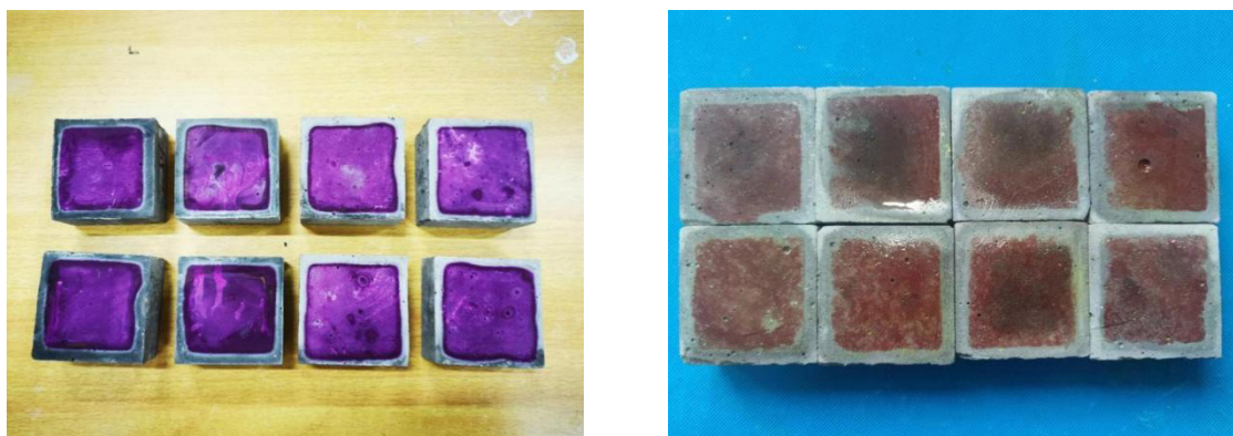
Fig. s3. Testing the depth of neutralization and chloride ion penetration
