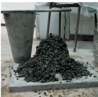
Fig. 12. Slump test of pervious concrete
