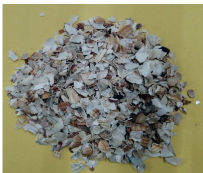
Fig. 1. Crushed shell aggregates
