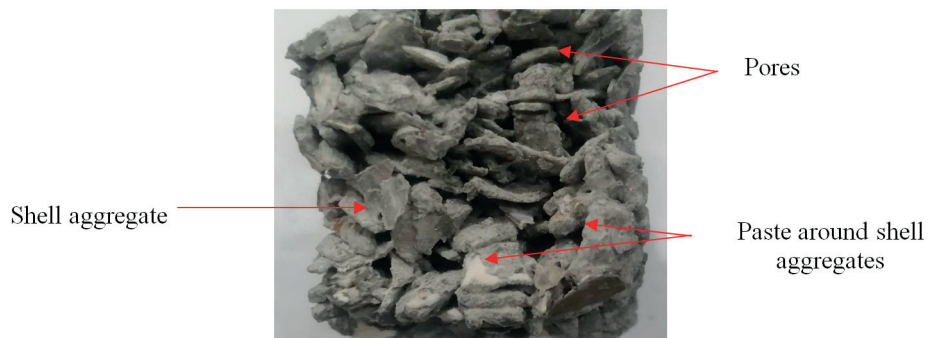
Fig.15. Porous texture of pervious concrete with shell aggregate
