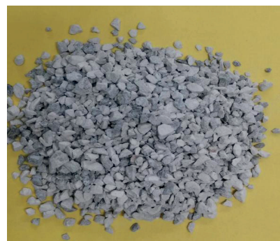
Fig. 2. Crushed limestone aggregates
