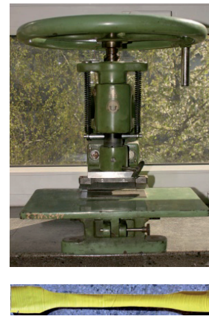
Fig. 2. Machine used for cutting out the samples and the picture of sample obtained
