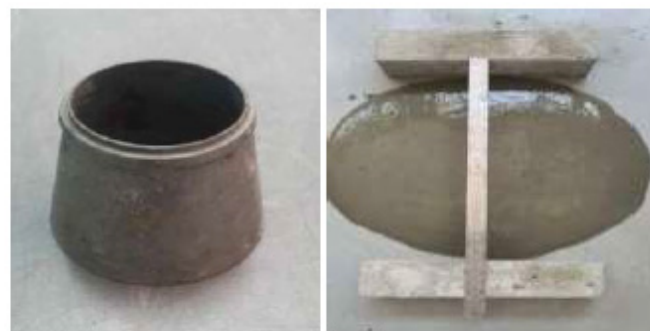
Fig. 4. Test to determine the spread at mini-slump cone.
